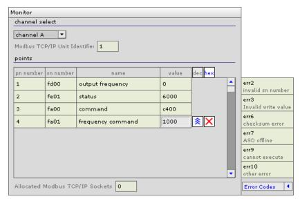
Figure 24: Embedded Web Server - edit point value & error code display
